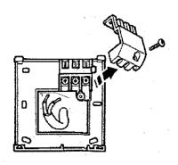
STEP 3: Remove battery shield to energize thermostat
